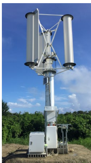
Magnus Vertical-Axis Wind Turbine set up in Nanjo, Okinawa Prefecture
